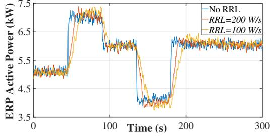
Fig. 6 Indicative ERP active power for different RRL levels
