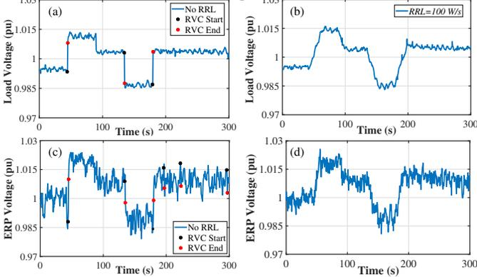
Fig. 7. Voltage profiles with respect to time: (a) Load Node Voltage - No RRL; (b) Load Node Voltage -  $RRL=100$  W/s; (c) ERP Node Voltage - No RRL; (d) ERP Node Voltage -  $RRL=100$  W/s
