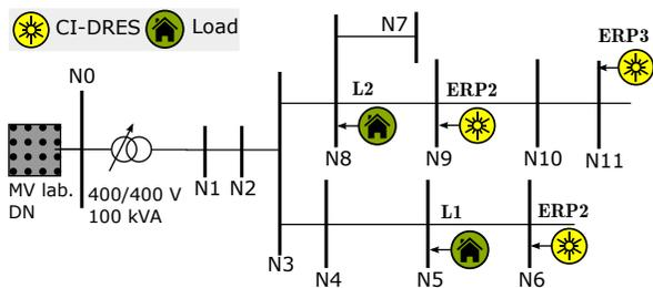
Fig. 4. Single-line diagram of the MV DN used for validation purposes, [20]. minimum voltage of the SC is 90 V. Hence, the total SC energy used for RRL control is equal to 9.33 Wh. A controllable current source emulates the primary energy source. The proposed control algorithm has been implemented in a Texas Instruments TMS320F28335 Delfino microcontroller with a sampling frequency of 20 kHz, thus 50  $\mu$ s sampling rate. More details can be found in [3], [22].
