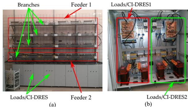
Fig. 5. Lab Scaled-down MV DN; (a) DN overview, (b) Cabinet interior
