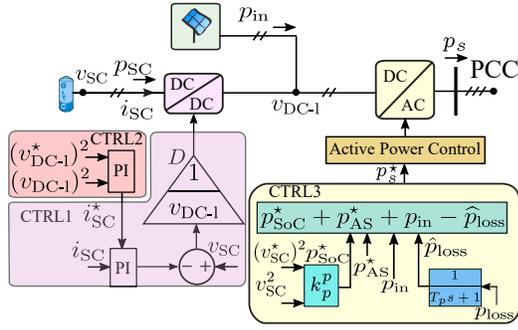
Fig. 2. Hierarchical CI-DRES control structure, [3], [22]
